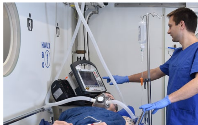
► With the HBO variant, the corpuls3 can be operated in multi-place hyperbaric chambers.
